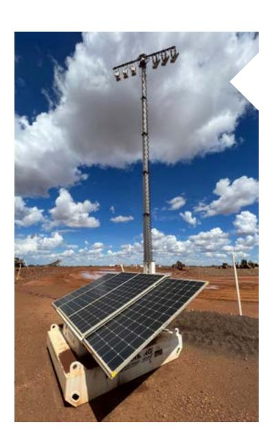
Thiess conducted solar lighting tower trials across multiple projects in Western Australia and Queensland. The plants saved on cost, diesel use and emissions while being virtually maintenance free, but challenges arose in terms of light output when compared to a diesel-powered equivalent. They have shared the learnings and other Thiess sites will investigate the applicability of solar lighting tower options in 2023.
