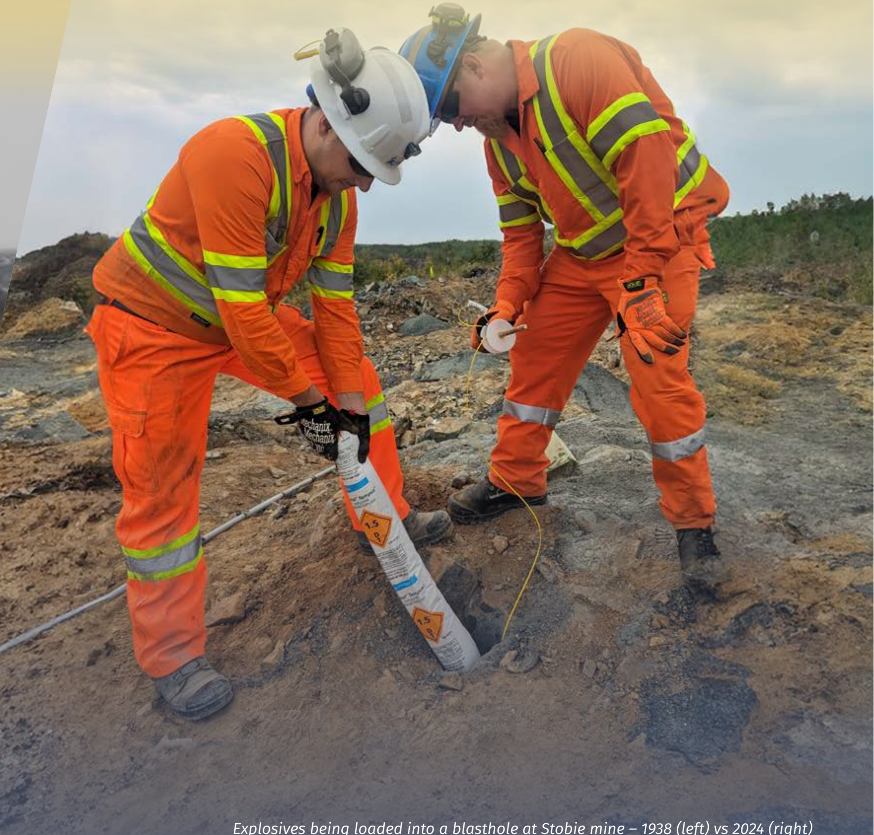
Explosives being loaded into a blasthole at Stobie mine – 1938 (left) vs 2024 (right)
